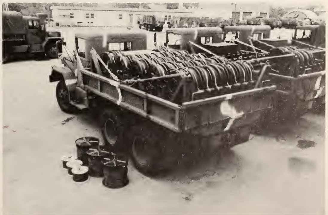
Fiber optic cable is much lighter and smaller. The three small rolls of fiber optic cable in the foreground replace the heavier copper cable carried by two and a half trucks.
