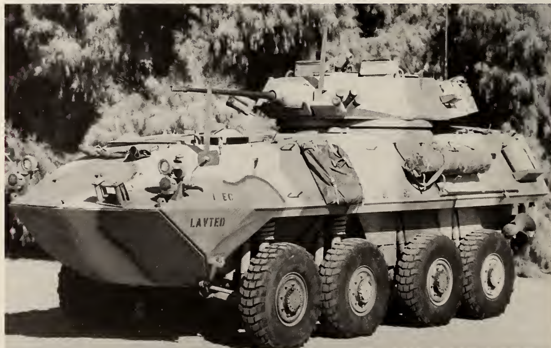
The basic LAV-25 (shown above) mounts an M242 25mm automatic cannon. The Air Defense and Assault Gun configurations will complete the LAV family which also includes Antitank, Mortar, Recovery, Command and Control, and Logistics variants.
